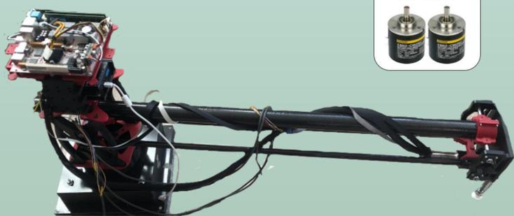
Complete design of one legged hopping robot
