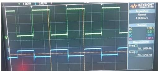
❖ Finally, the other Arduino converts the serial data bundle to PWM. We pass the converted signal through a lowpass filter and through an audio amplifier. Then we get final result shown in below;
