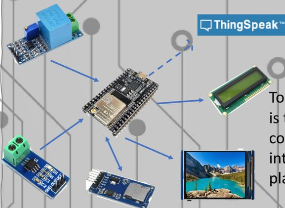
Today, the internet is at the center of life in a location that everyone can easily access and use. While this is the case, we technology developers must provide access to the internet in our projects. By connecting the test and measurement integrated device for the AC motors we have built to the internet, we have enabled users to access the data online. We published the data on the ThingSpeak platform, which is frequently used by IoT developers, with the WiFi module included in the ESP32.
