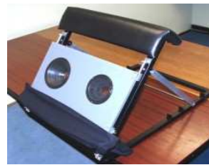
Figure 18: Fibre holder rings and support frame for optical tomography of the breast ([3])
