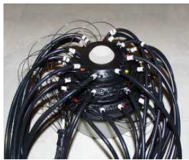
Figure 19: Source and detector fibres attached to three rings mounted on a conical phantom ([3])
