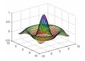
produces a surface with a face alpha value of 0.4. Alpha values range from 0 (completely transparent) to 1 (not transparent).
