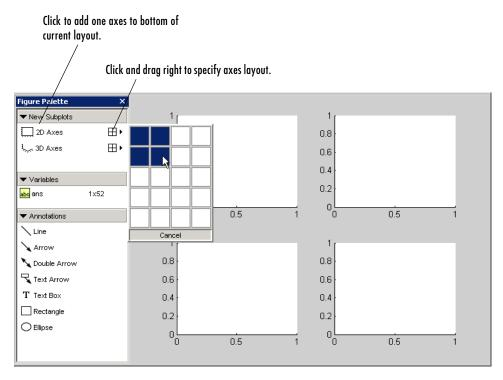
Select the axes you want to target for plotting. You can also use the subplot command to create multiple axes.
