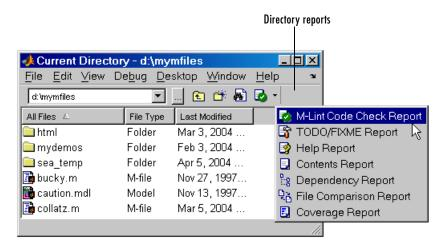
In MATLAB, the M-Lint Code Check Report displays a message for each line of an M-file it determines might be improved. For example, a common M-Lint message is that a variable is defined but never used in the M-file.
