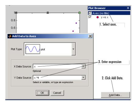
The picture above shows how to configure the Add Data to Axes dialog to create a line plot of  $y = x^4$ , which is added to the existing plot of  $y = x^3$ .
