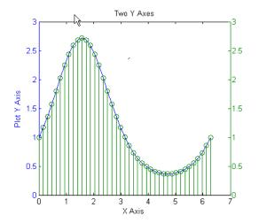
This graph contains two *y*-axes, one for each plot type (lineseries and stem graphs). The plotting tools make it easy to select any of the objects that the graph contains and set their properties.
