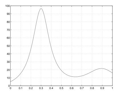
The graph shows that the function has a local minimum near x = 0.6. The function fminsearch finds the *minimizer*, the value of x where the function takes on this minimum. The first argument to fminsearch is a function handle to the function being minimized and the second argument is a rough guess at the location of the minimum:
