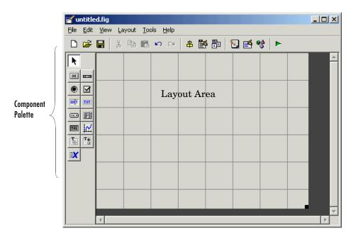
You can lay out your GUI by dragging components, such as panels, push buttons, pop-up menus, or axes, from the component palette, at the left side of the Layout Editor, into the layout area. For example, if you drag a push button into the layout area, it appears as in the following figure.
