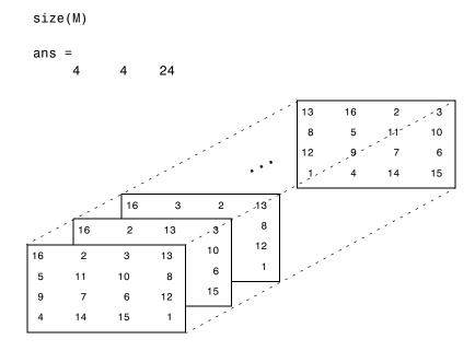
stores the sequence of 24 magic squares in a three-dimensional array,  $\ensuremath{\mathsf{M}}.$  The size of  $\ensuremath{\mathsf{M}}$  is
